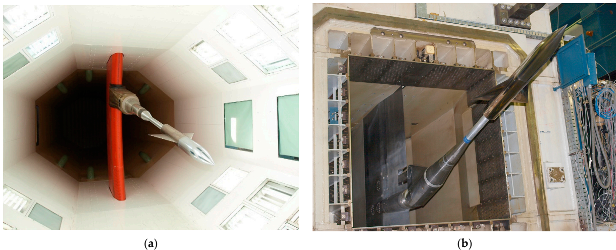
Figure 7. The 115.8 mm diameter AGARD-B standard model: (a) the model in the test section of the T-35 wind tunnel [44]; (b) the model in the test section of the T-38 wind tunnel.
