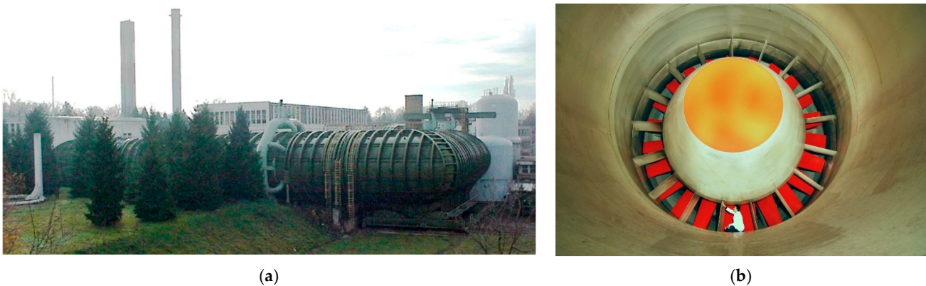
Figure 3. The T-35 subsonic wind tunnel of VTI: (a) external view; (b) the variable-pitch fan blades of T-35 [44].
