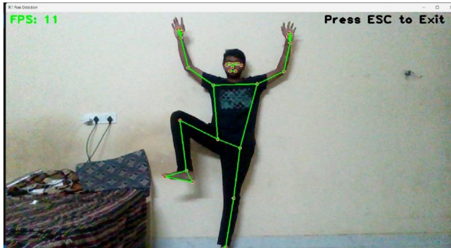
Fig. 3. Landmark Detection and tracking using Mediapipe
